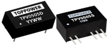
**DESCRIPTION: 1W 3KVDC Isolated Single & Dual Output DC/DC Converters**
